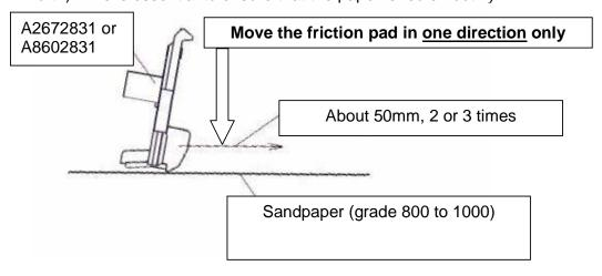
After smoothing out the pad surface, check the paper feed with a full paper tray.
